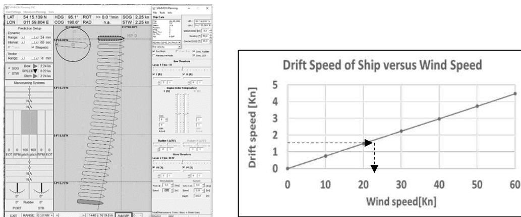
Figure 2: Transverse Drifting under Wind speed  $V_A=30\text{kn}$  (Cruise ship AIDAblu). Left: situation with drift speed  $SOG=2.25\text{kn}$ ,  $HDG\ 94^\circ$ ,  $COG\ 184^\circ$ ; right: diagram for drift speed versus wind speed with arrows indicating maximum drift balance by thrusters
