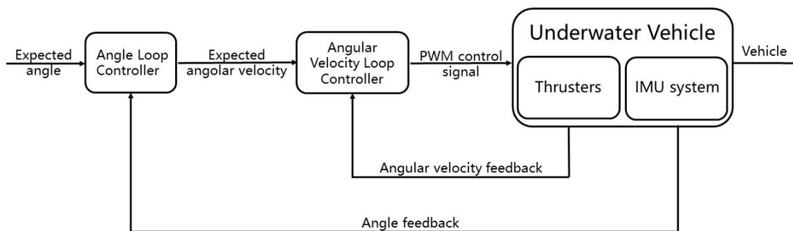
**Figure 4.** Structure of multi-stage angular PID controller
