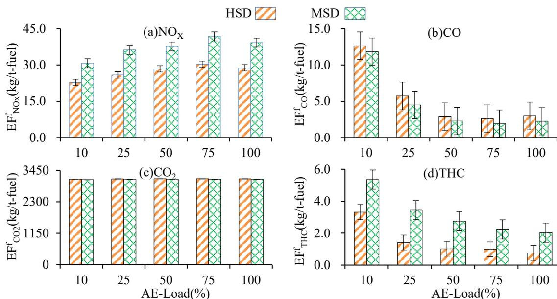
Figure 3. AE's fuel-based emission factors under different load
