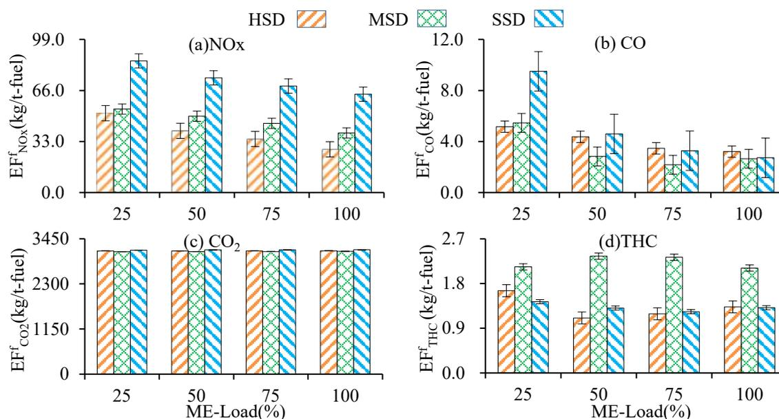
Figure 2. ME's fuel-based emission factors under different load
