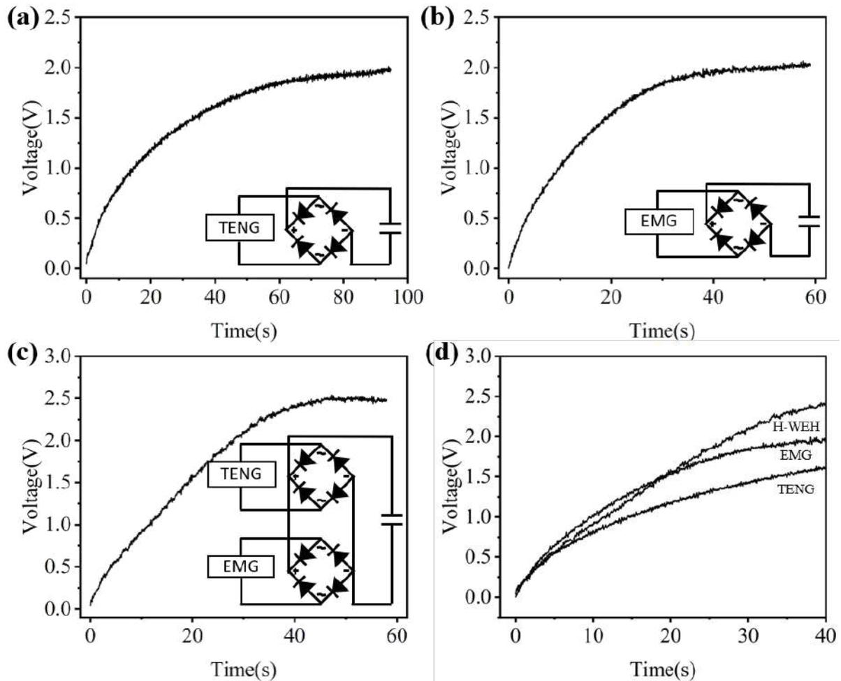
**Figure 4.** (a) Voltage curves of a capacitor charged by the TENG component. (b) Voltage curves of a capacitor charged by the EMG component. (c) Voltage curves of a capacitor charged by H-WEH. (d) Charging curves of a capacitor using TENG only, EMGs, and the H-WEH.
