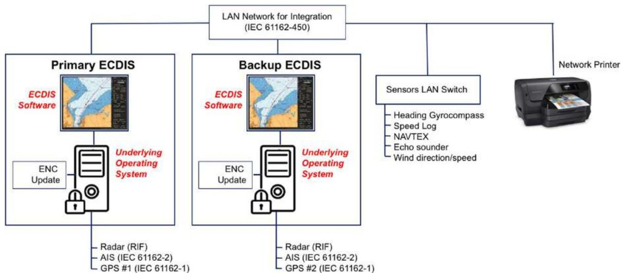
**Figure 1:** Primary and backup ECDIS arrangement
