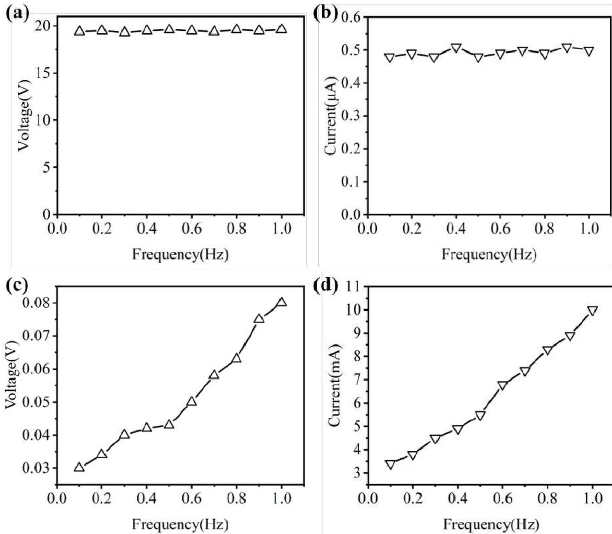
**Figure 2.** H-WEH output characteristics at different frequencies. (a) The voltage of the TENG component at different frequencies. (b) The Current of the TENG component at different frequencies. (c) The voltage of the EMG component at different frequencies. (d) The current of the EMG component at different frequencies.
