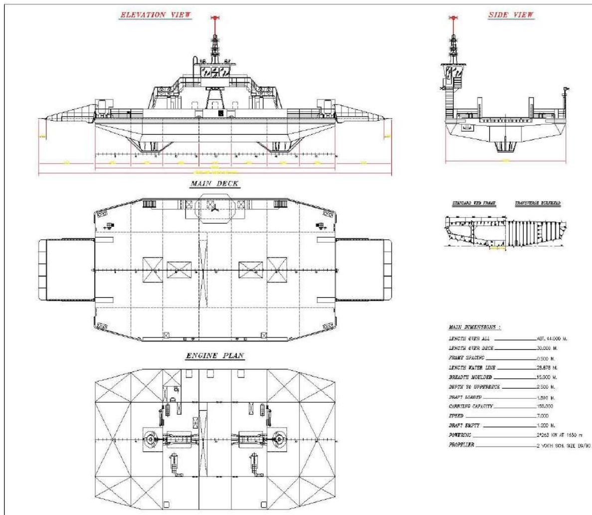
Figure 1 General arrangement of the car/passenger ferry
