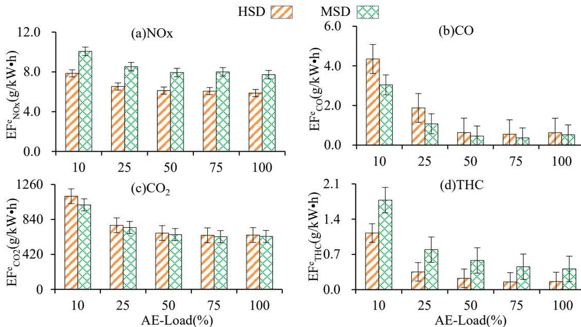
Figure 5. AE's energy-based emission factors under different load
