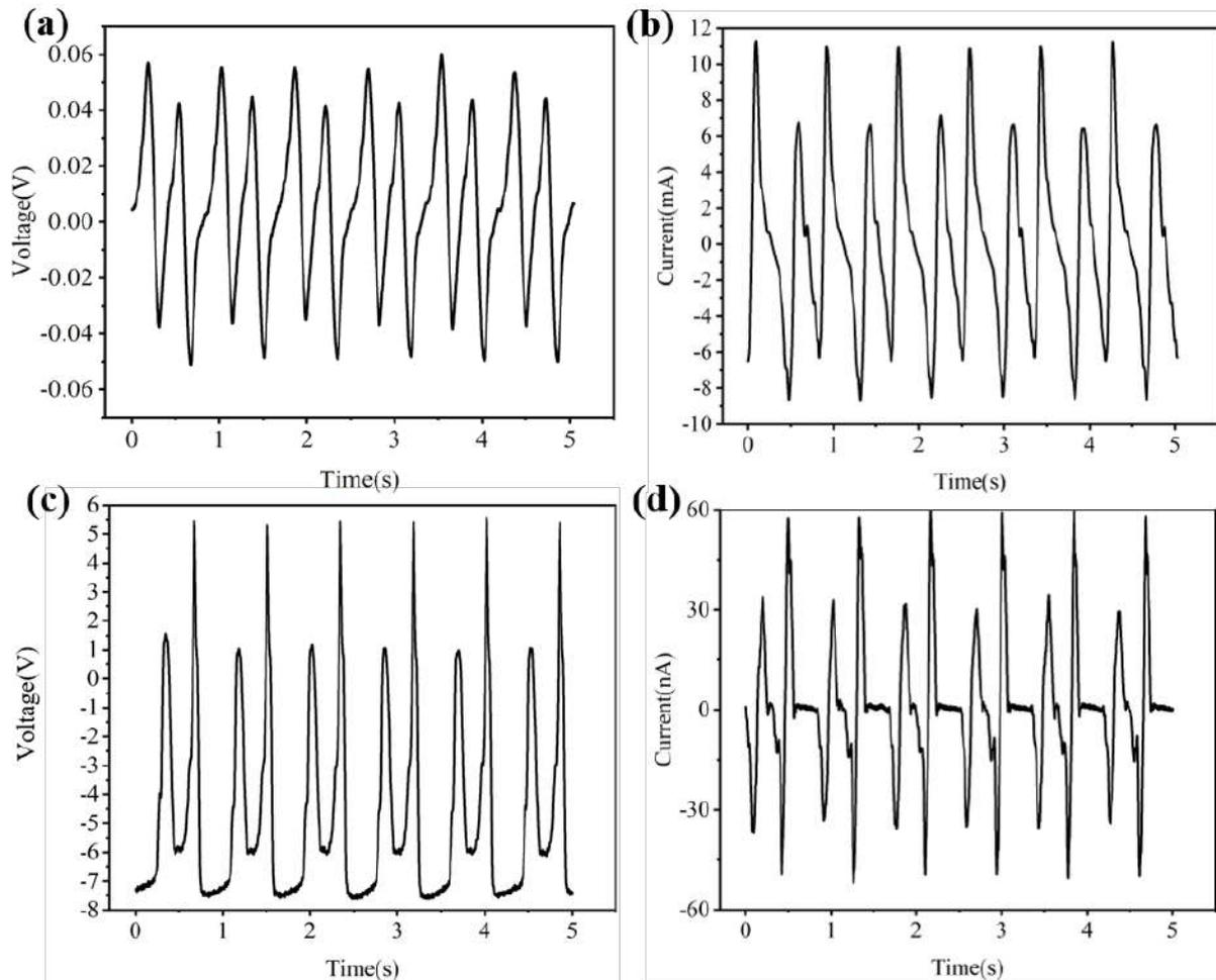
**Figure 3.** The output characteristics of H-WEH under the excitation of waves with a frequency of 1Hz and a height of 5CM. (a) TENG's voltage curve. (b) TENG's current curve. (c) EMG's voltage curve. (d) EMG's current curve.
