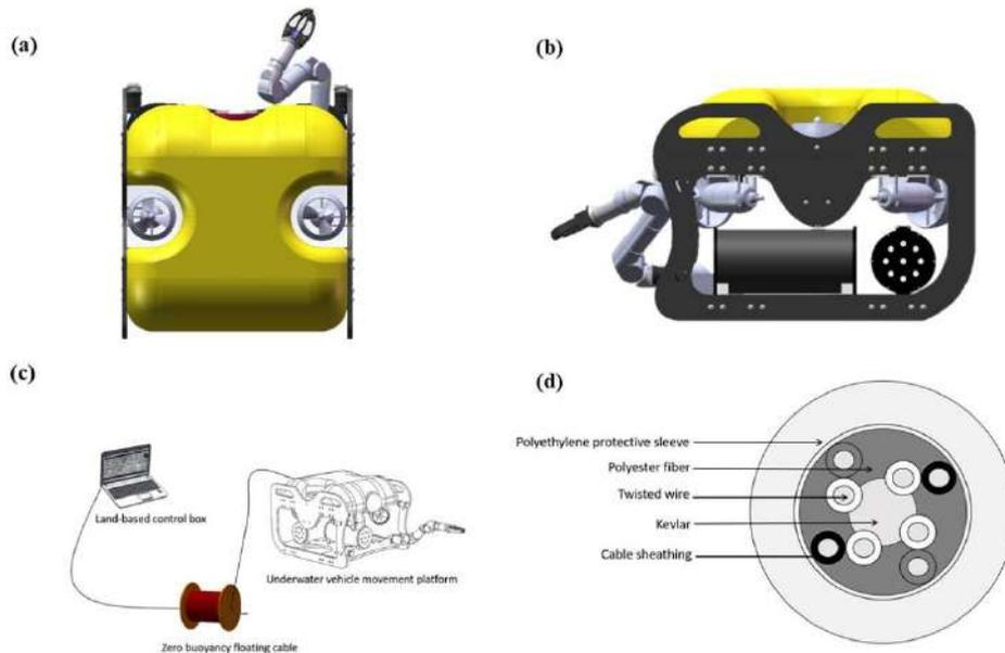
**Figure 2.** Underwater intelligent robot system architecture. (a) Top view of the underwater vehicle body motion platform; (b) Side view of the underwater vehicle body motion platform; (c) General framework of underwater intelligent vehicle system; (d) Zero buoyancy cable structure
