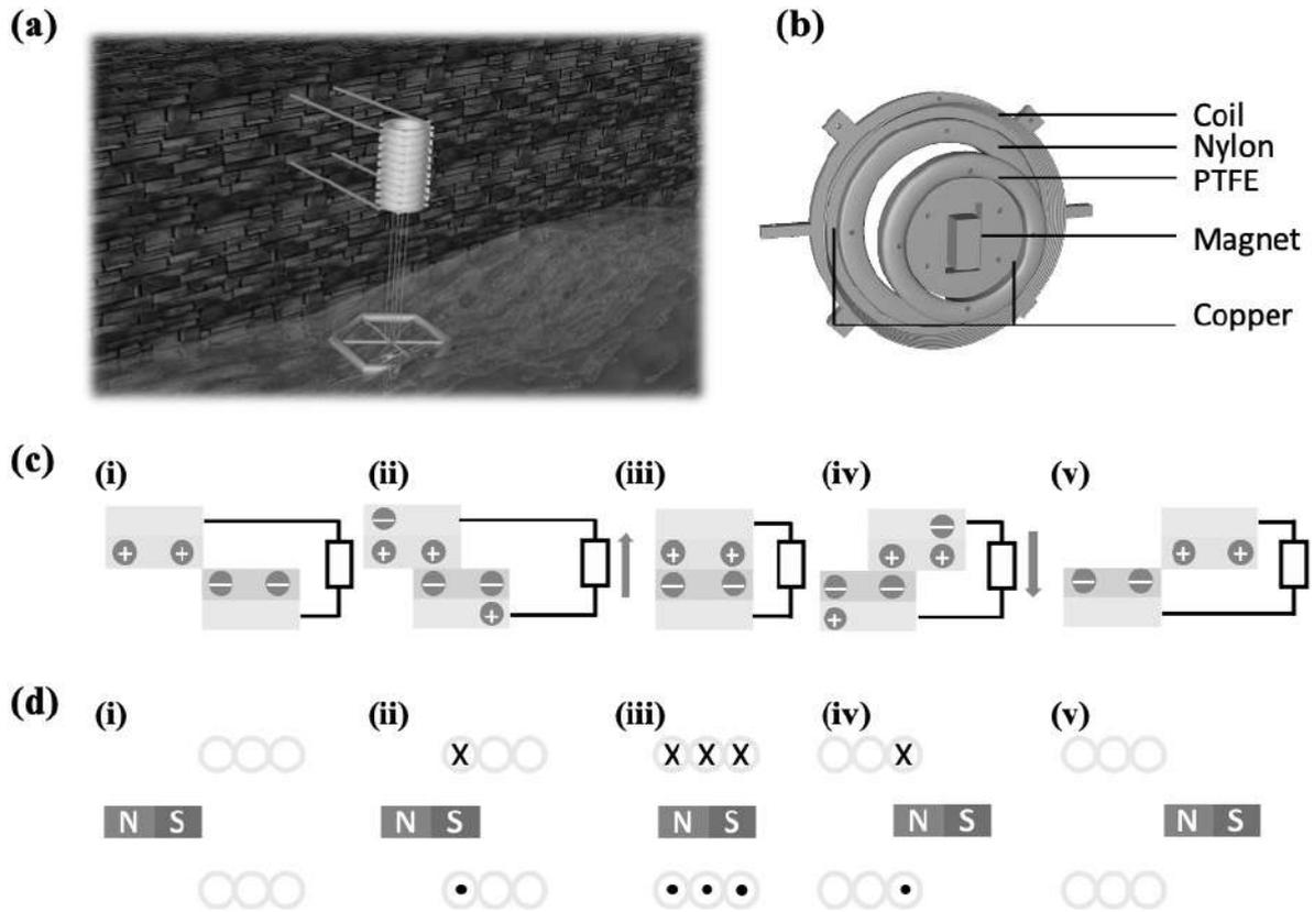
**Figure 1.** Structural design and working principles of the T-TENG. (a) Schematic diagram of the designed H-WEH consisting of multiple units. (b) Exploded view of the H-WEH's structure. (c) The working principle of the TENG component. (d) The working principle of the EMG component.
