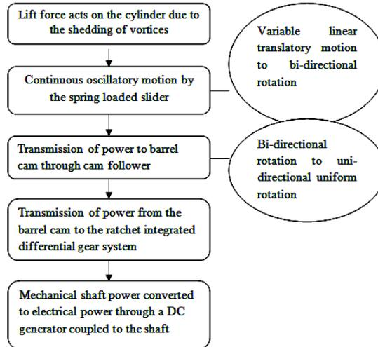
Fig.2. Flow diagram of power transmission system
