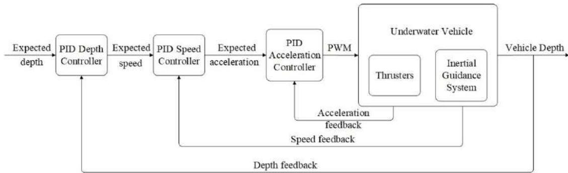
**Figure 6.** Structure of depth loop PID controller
