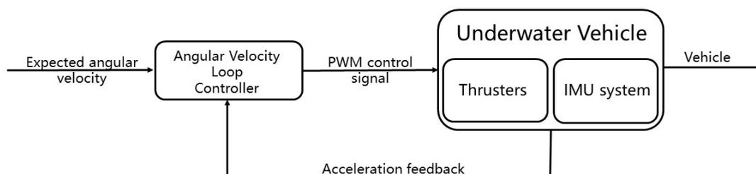
**Figure 5.** Structure of single-stage angular velocity PID controller
