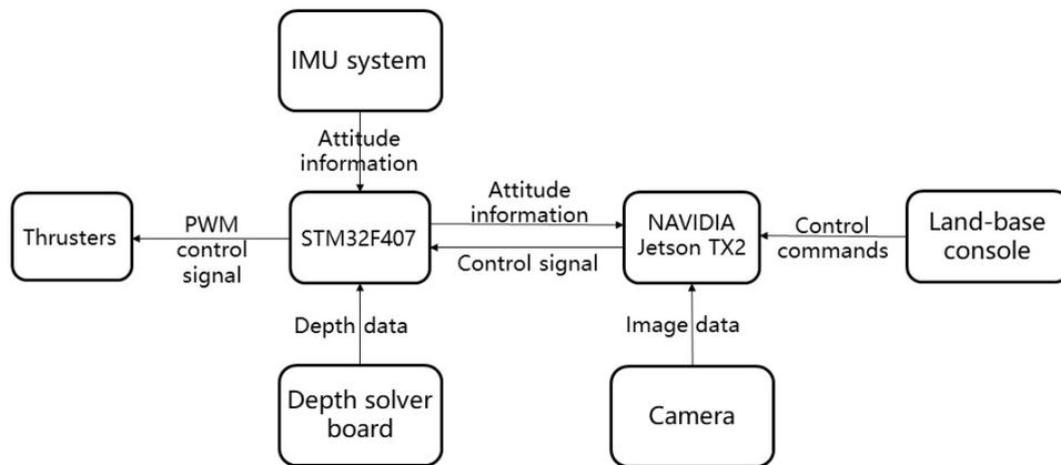
**Figure 3.** Underwater vehicle control system design block diagram
