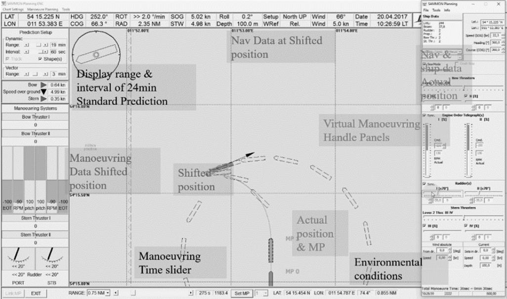
Figure 1: Interface elements of SAMMON Manoeuvring Design & Planning tool with additional comments (more information under YouTube [7])
