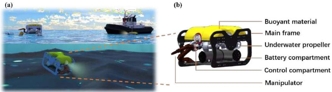
**Figure 1.** Application of marine environment perception underwater vehicle system and architecture. (a) Multiple application scenarios of marine environmental perception underwater vehicle systems; (b) Underwater vehicle architecture.
