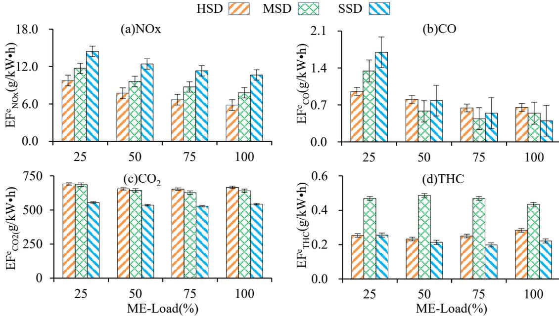
Figure 4. ME's energy-based emission factors under different load
