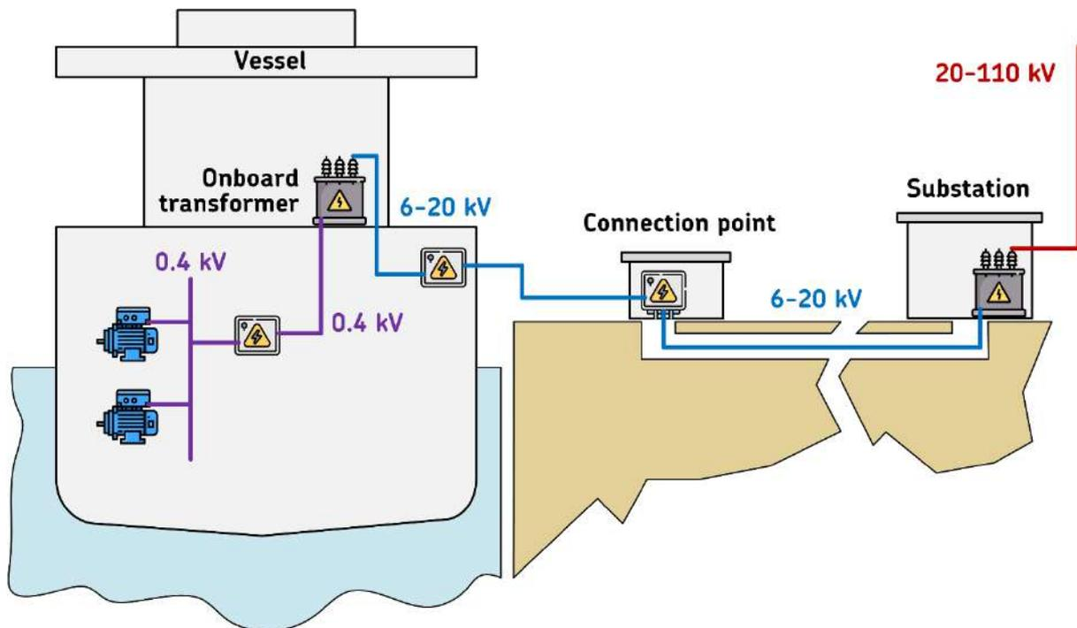
Figure. 1. General arrangement of cold ironing [2][1].
